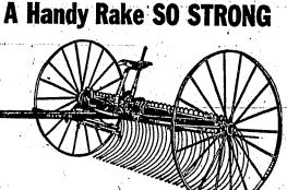
This is the Oliver Sulky Dump Rake. Its bridge-trussed frame prevents sagging and twisting and has a reputation
