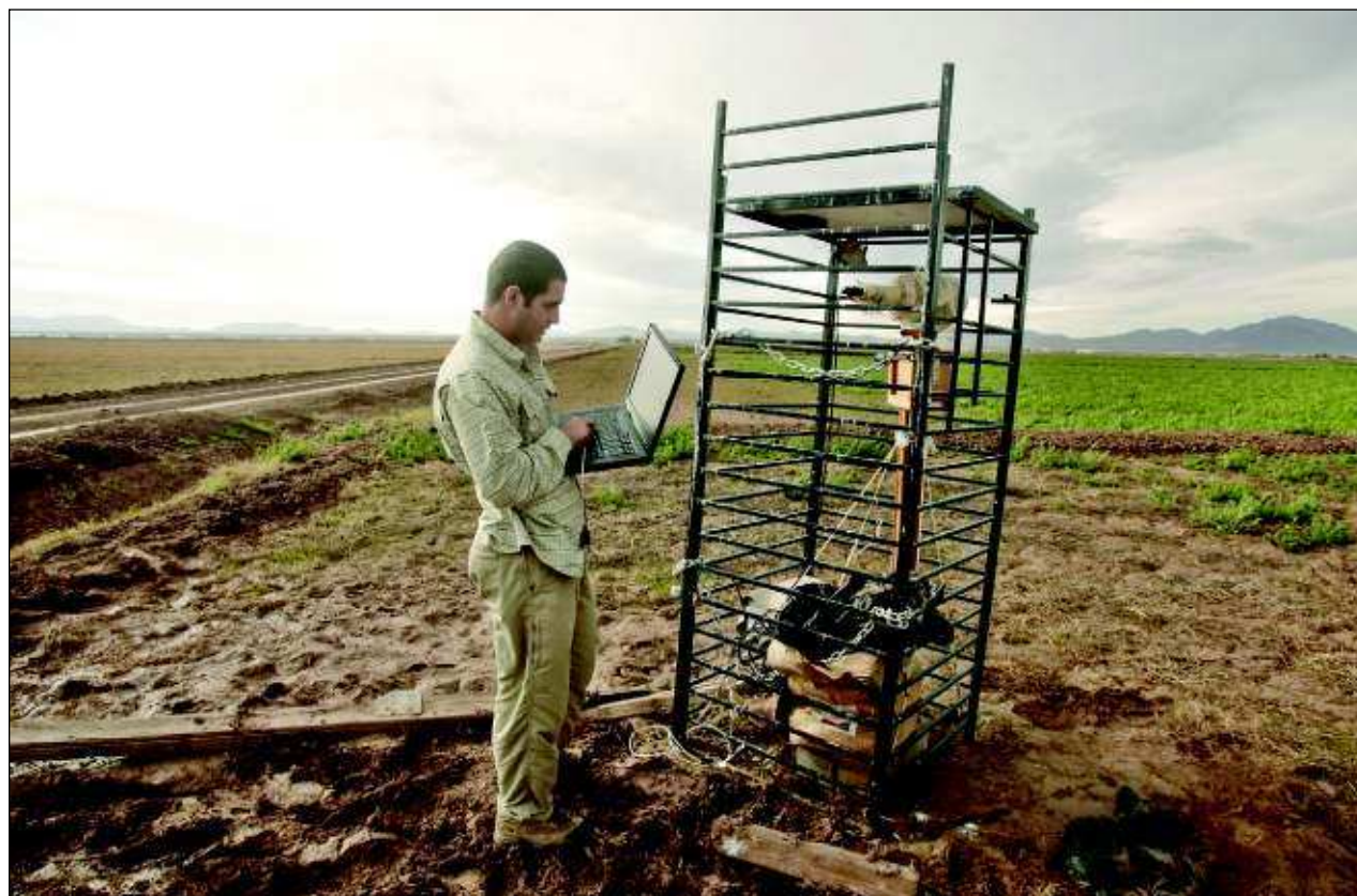
Samer Naif, a student at the University of California San Diego, connects his laptop to a scintillometer receiver in an alfalfa field in Blythe, Calif. It's a laser device that measures evaporation and helps in calculating exactly how much water is needed to properly irrigate. AP photo
