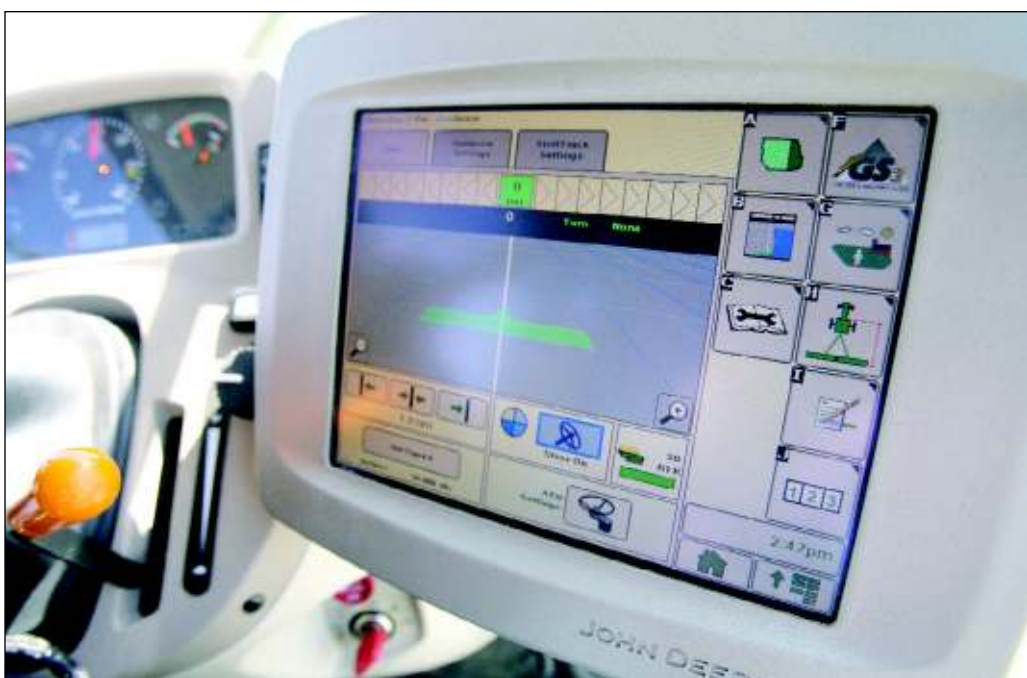
A close up view of the GS2 system that utilizes GPS and GIS technology to eliminate 'guess rows.'
