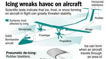
Deflate mounted on the wing's leading edge, expand like balloons to pop off ice.
