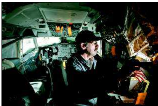
Mechanic Richard Robertson works on a Boeing 727. Preparing planes for storage — taking them apart and draining their fluids — is called 'pickling.'
