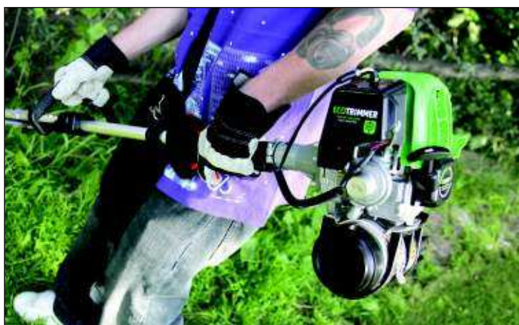
The Lehr Eco Trimmer uses a propane canister to fuel its 25-cc, four-stroke engine.
