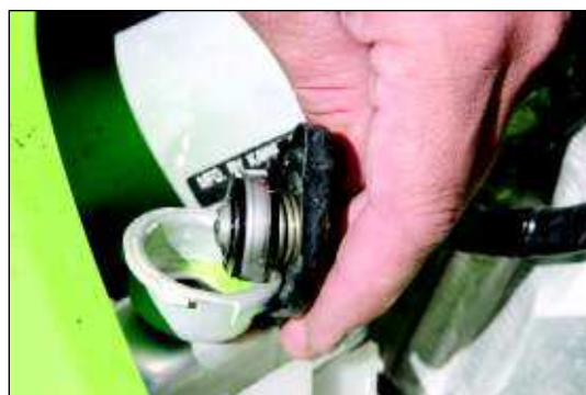
Riders should make sure their liquid-cooled machines have antifreeze that's 'up to snuff' as the the cold months approach, Jamey Wills says. 'Make sure your antifreeze has a freeze rating of 30 below,' he says.
