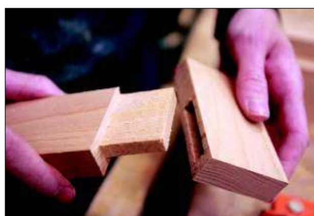
A mortise and tenon joint that Brian Cotton is using in his bookshelf.
