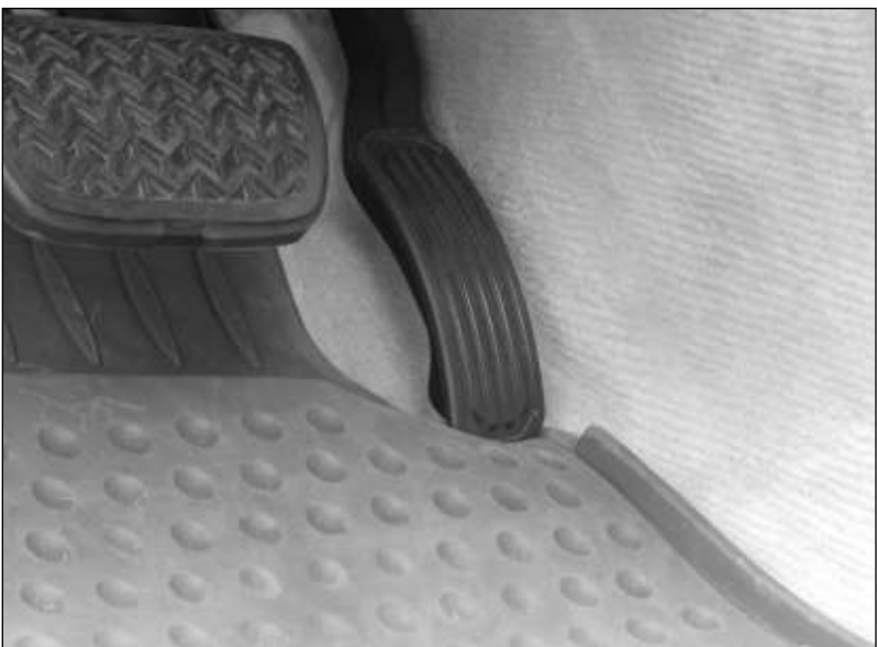
This undated photo provided by the National Highway Traffic Safety Administration shows an unsecured driver's-side floor mat trapping the accelerator pedal in a 2007 Lexus ES350. NHTSA/AP photo
