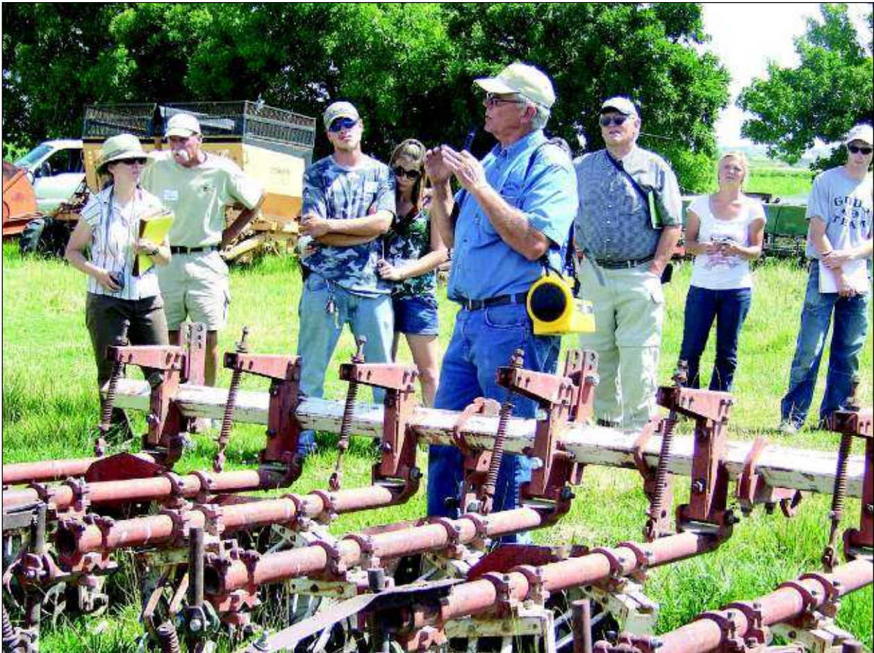
CINDY SNYDER/For the Times-News Mike Heath explains how his father-in-law, who owned a blacksmith shop in Buhl, converted old grain drills into bean planters. Even though it's not a precision planter by today's standards, these old planters are easy to adjust and are still available.
