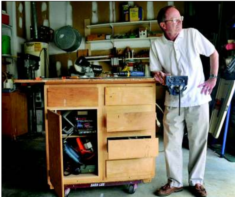
Nathan Gilbert with his portable workbench. Gilbert didn't have any room in his garage for a permanent workbench, so he screwed together a couple of kitchen cabinets and put them on casters.
