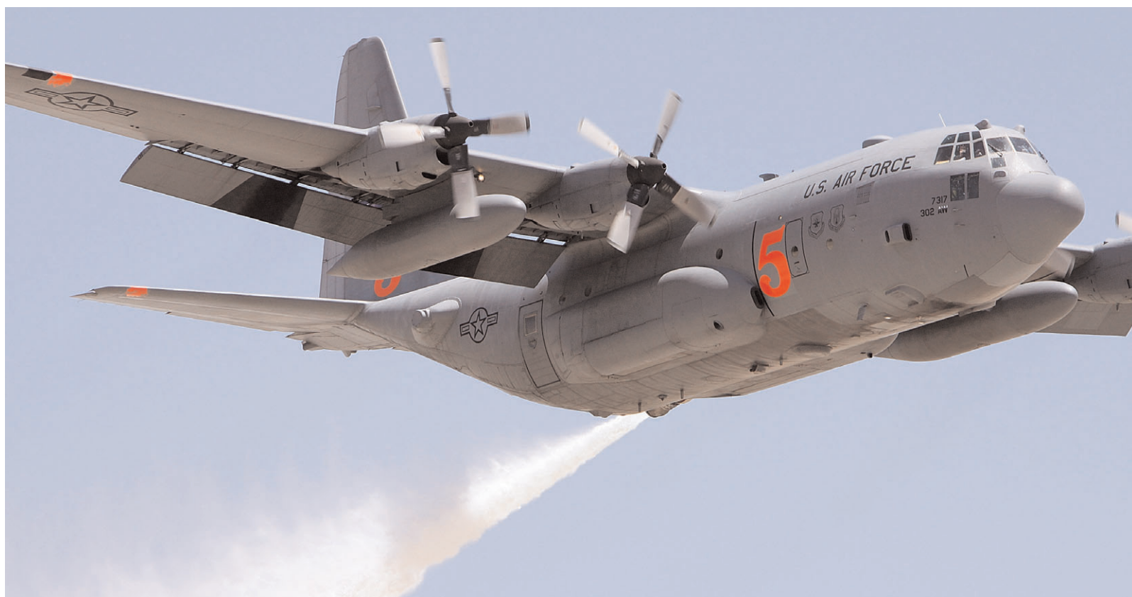
A Colorado Reserve C-130 drops water on a target in 2009 during a certification flight at the Tucson International Airport in Tucson, Ariz. Military cargo planes used to drop slurry on wildfires are now based in Utah and Idaho.
