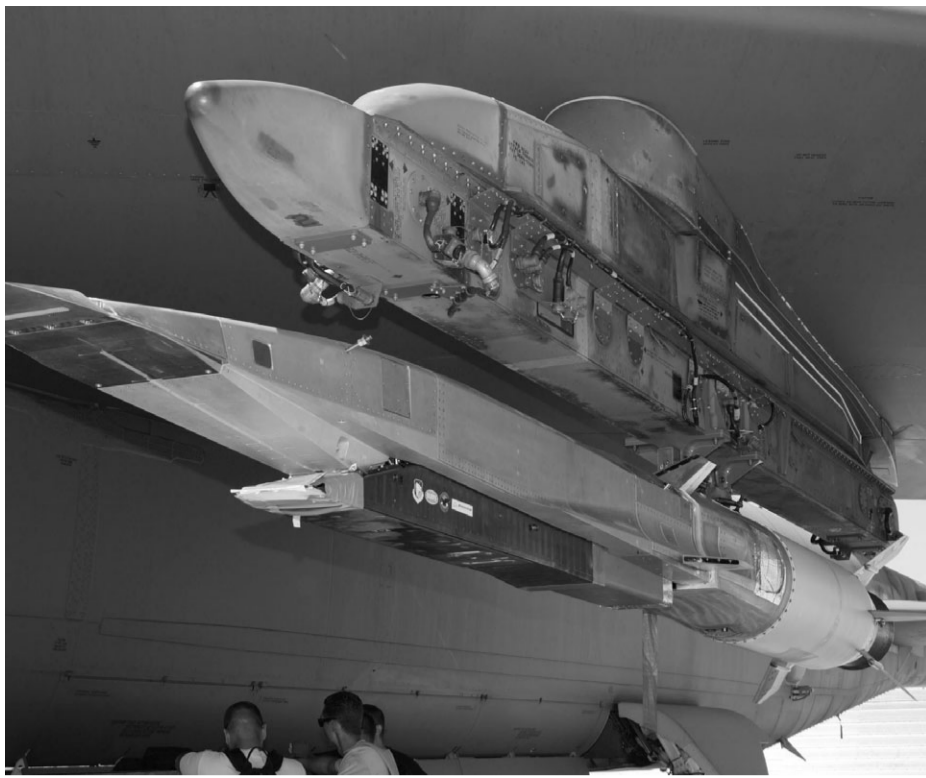
The X-51A WaveRider hypersonic flight test vehicle is uploaded to an Air Force Flight Test Center B-52 for fit testing in 2009 at Edwards Air Force Base.
