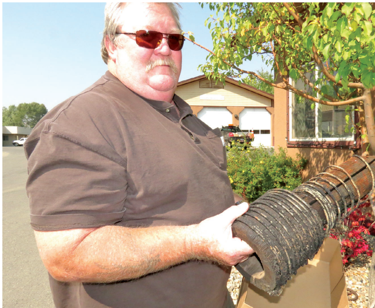
Dave Rambo, Ketchum's water division supervisor, shows off a piece of redwood pipe that was considered state-of-the-art when it was laid as water pipe under Ketchum.
