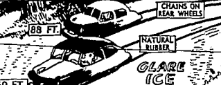
The chains are the most effective self-help for the motorist in increasing traction on icy and snowy surfaces. Remember that chains do not provide steering control so necessary on curves.
