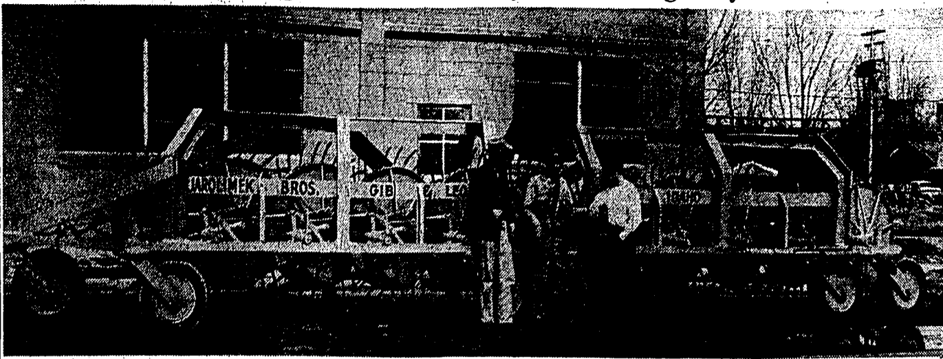
Probably the largest of its kind, the sagebrush rake pictured above, owned by Jarolmek brothers Sagebrush Land Clearing service, Filer, is scheduled for work on the Mindoka reclamation project this week as construction was completed by the Acme Machine works, Filer. The six-ton behemoth, equipped with hydraulic steering, rakes a swath 20 feet wide and is pulled by a D-6 caterpillar. The rake was finished by the Filer firm just two and one-half weeks after work began, and although a few of the basic parts are copied, most of the machine was conceived and made by the Filer mechanics. It is capable of clearing from 75 to 100 acres in an eight hour day. Above, Gilbert Jarolmek, left, and Leo Jarolmek, right, look over the machine with William Herrett, center, owner of the Acme Machine shop. (Staff photo-engraving)
