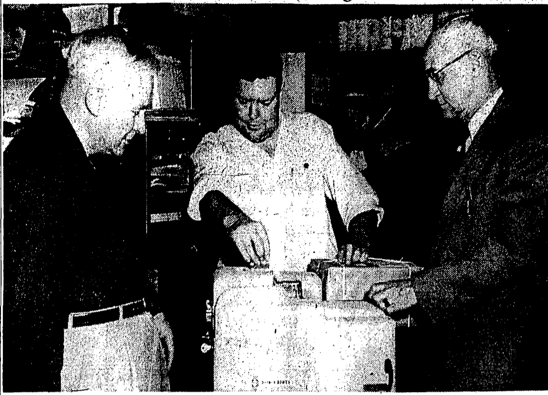
The Twin Falls postoffice's new postage meter machine, shown above, is expected not only to save time for the patron but time and money for the government. The electrically operated mechanism automatically registers the postage charge and cancellation upon the press of a button. Above, Hubert Williams, parcel post window clerk, center, prepares to affix one of the printed labels to a package under the supervision of A. T. Anderson, superintendent of mails, left and Postmaster W. W. Frantz. (Staff photo-engraving)
