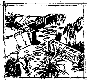
This type of structure is gaining in popularity because of its ease of construction and low cost. The 2x2 inch slotted blocks have to be specially ordered at the present time.
