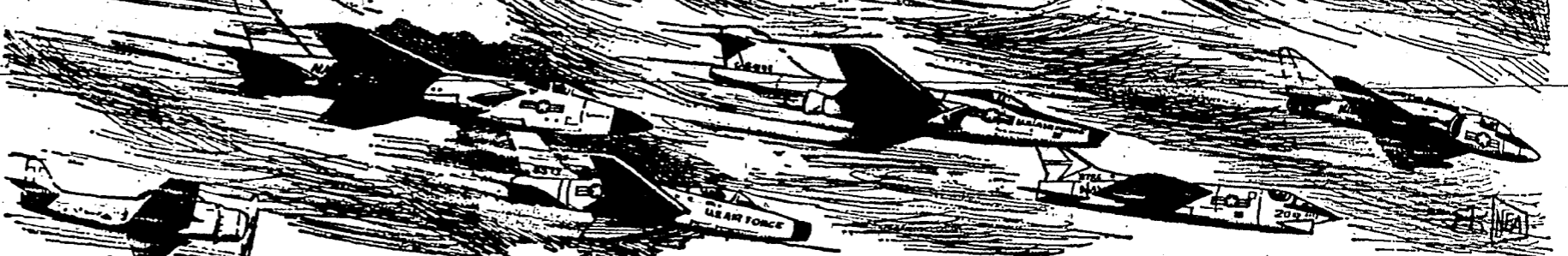
A1-E SKYRAIDER Prop-driven all-purpose craft used by South Vietnamese R4SC VIGILANTE Navy carrier-based fighter-bomber F-100 SUPERSABRE Air Force fighter-bomber RF-101 VOODOO Air Force photo-reconnaissance fighter F8U CRUSADER Navy carrier-based fighter A4D2 SKYHAWK Navy carrier-based attack bomber
